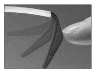
LIVING HINGE - Multiple materials have been laid simultaneously in an additive manufacturing method using the Connex 500™ from Object to mimic a living tooling.
